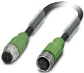
Sensor/actuator cable, 5-position, PUR halogen-free, black-gray RAL 7021, shielded, Plug straight M12, A-coded, on Socket straight M12, A-coded, cable length: 10 m
