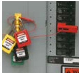
Step 4: For group lockouts, run key through multiple loops in lock rail and apply the locks. No hasps required!
