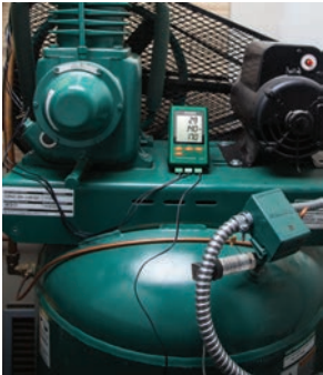
SD750 3-Channel Pressure Meter/Datalogger (p. 109)
