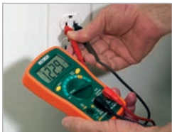
Displays AC Voltage of an outlet receptacle
