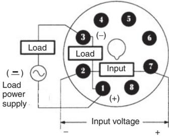
Note: The symbols shown in parentheses are for DC loads. The load is possible to connect either + side or - side.
