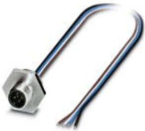
Flush-type connector, 4-position, Plug, M12, A - standard, Front mounting, M20 x 1,5, Individual wires, cable length: 0.5 m, 0.34 mm 2 , TPE litz wire
