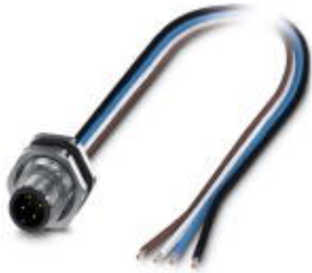
Flush-type connector, Universal, 4-position, Plug, M12, A-coded, Rear mounting, M16 x 1.5, Individual wires, cable length: 0.5 m
