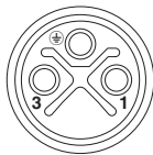
Pin assignment of M12 socket, 3-pos., S-coded, socket side view
