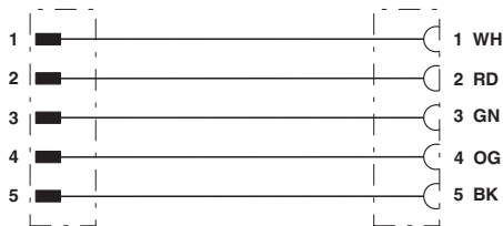
Contact assignment of 7/8" plugs/sockets
