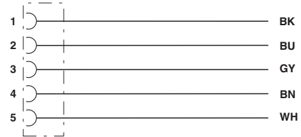
Contact assignment of 7/8" socket
