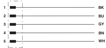
Contact assignment of 7/8" plug
