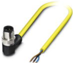
Sensor/actuator cable, 3-position, PVC, Plug angled M12 SPEEDCON, A-coded, on free cable end, Cable length: 2 m
