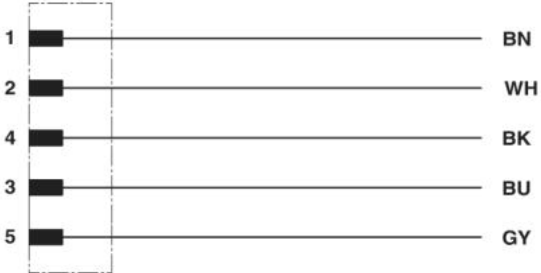
Contact assignment of the M12 plug
