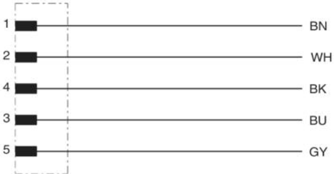
Contact assignment of the M12 plug
