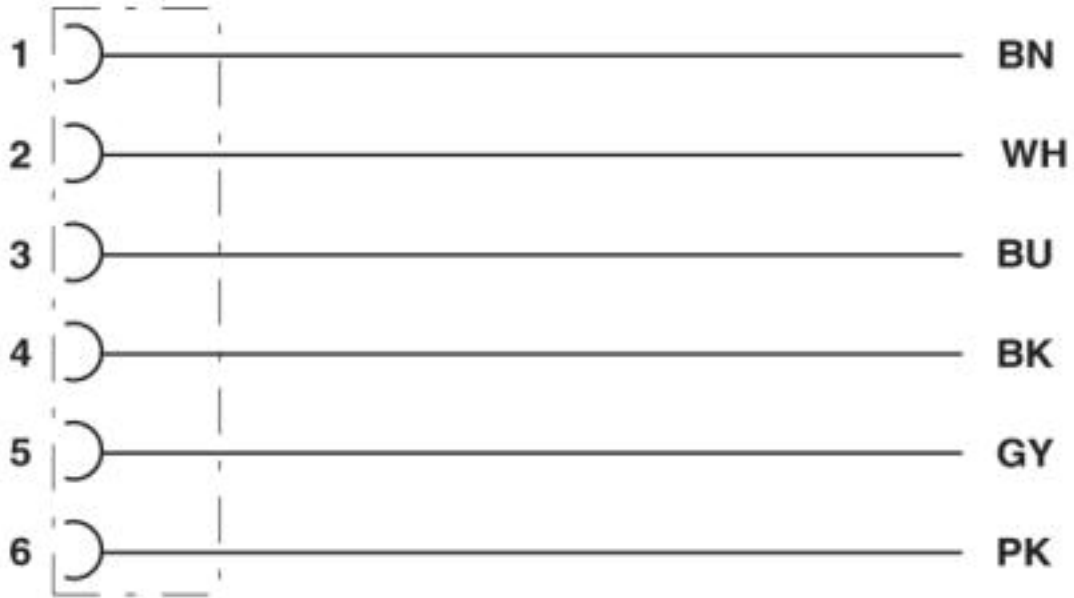
Contact assignment of M8 socket
