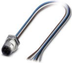
Sensor/actuator flush-type male connector, 5-pos., M12 SPEEDCON, B-coded, rear/screw mounting with M12 thread, with 0.5 m TPE litz wire, 5 x 0.34 mm 2
