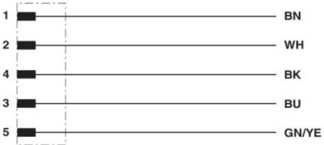
Contact assignment of the M12 plug
