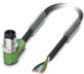
Sensor/actuator cable, 5-position, Variable cable type, Plug angled M12, A-coded, on free cable end, cable length: Free input (0.2 ... 40.0 m)
