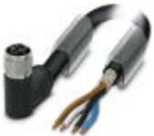
Power cable, 4-position, PUR halogen-free, black RAL 9005, shielded (Advanced Shielding Technology), free cable end, on Socket angled M12, T-coded, cable length: 1.5 m, For direct current up to 12 A/63 V
