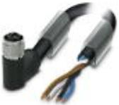
Power cable, 4-position, PUR halogen-free, black-gray RAL 7021, free cable end, on Socket angled M12, T-coded, cable length: 1 m, For direct current up to 12 A/63 V
