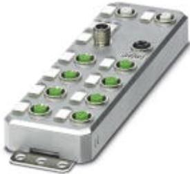
Axioline E, Digital input device, Sercos, M12 fast connection technology, Digital inputs: 16, 24 V DC, connection method: 4-wire, Metal housing, degree of protection: IP65/IP67
