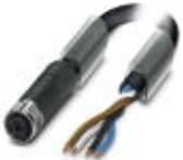
Power cable, 4-position, PUR halogen-free, black-gray RAL 7021, free cable end, on Socket straight M12, T-coded, cable length: 1 m, For direct current up to 12 A/63 V
