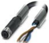
Power cable, 4-position, PUR halogen-free, black-gray RAL 7021, free cable end, on Socket straight M12, T-coded, cable length: 5 m, For direct current up to 12 A/63 V
