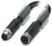
Power cable, 4-position, PUR halogen-free, black-gray RAL 7021, Plug straight M12, T-coded, on Socket straight M12, T-coded, cable length: 1 m, For direct current up to 12 A/63 V
