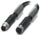
Power cable, 4-position, PUR halogen-free, black-gray RAL 7021, Plug straight M12, T-coded, on Socket straight M12, T-coded, cable length: 2 m, For direct current up to 12 A/63 V
