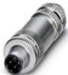
Bus system connector, Ethernet/PROFINET CAT5 (100 Mbps), 4-position, shielded, Plug straight M12, D-coded, Screw connection, knurl material: Zinc die-cast, nickel-plated, cable gland Pg9, external cable diameter 6 mm ... 8 mm
