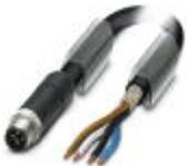
Power cable, 4-position, PUR halogen-free, black RAL 9005, shielded (Advanced Shielding Technology), Plug straight M12, T-coded, on free cable end, cable length: 1.5 m, For direct current up to 12 A/63 V
