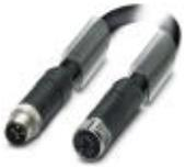
Power cable, 4-position, PUR halogen-free, black-gray RAL 7021, Plug straight M12, T-coded, on Socket straight M12, T-coded, cable length: 0.6 m, For direct current up to 12 A/63 V
