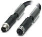
Power cable, 4-position, PUR halogen-free, black-gray RAL 7021, Plug straight M12, T-coded, on Socket straight M12, T-coded, cable length: 0.3 m, For direct current up to 12 A/63 V
