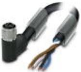
Power cable, 4-position, PUR halogen-free, black-gray RAL 7021, Socket angled M12, on free cable end, cable length: 5 m, For direct current up to 12 A/63 V
