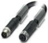
Power cable, 4-position, PUR halogen-free, black-gray RAL 7021, Plug straight M12, T-coded, on Socket straight M12, T-coded, cable length: 5 m, For direct current up to 12 A/63 V
