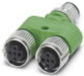
Y distributor, 5-position, Plug straight M12 SPEEDCON, A-coded, on Socket straight M12 SPEEDCON, A-coded and Socket straight M12 SPEEDCON, A-coded, Parallel distributor, Thread M12 socket not rotatable
