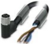
Power cable, 4-position, PUR halogen-free, black-gray RAL 7021, Socket angled M12, on free cable end, cable length: 10 m, For direct current up to 12 A/63 V
