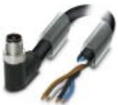
Power cable, 4-position, PUR halogen-free, black-gray RAL 7021, Plug angled M12, T-coded, on free cable end, cable length: 1 m, For direct current up to 12 A/63 V
