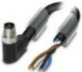
Power cable, 4-position, PUR halogen-free, black-gray RAL 7021, Plug angled M12, T-coded, on free cable end, cable length: 10 m, For direct current up to 12 A/63 V
