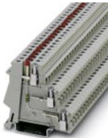
Sensor/actuator terminal block, Cross section: 0.2 mm 2 - 4 mm 2 , AWG: 24 - 12, Connection type: Screw connection, Width: 6.2 mm, Color: gray, Mounting type: NS 35/7,5, NS 35/15
