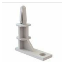
PCB Support, Top Hole: Snap Lock .125 in/ .062 in Panel, Bottom Hole: #4; M3 Hole, Natural, UL94 V-2 Nylon 6/6
