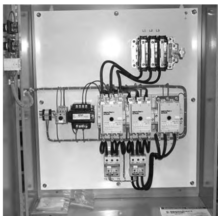
Custom 2-speed, 1-winding combination starter with control transformer and deceleration relay, mounted in a Type-1 enclosure
